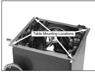
Figure 25. Table mounting bolt holes.
